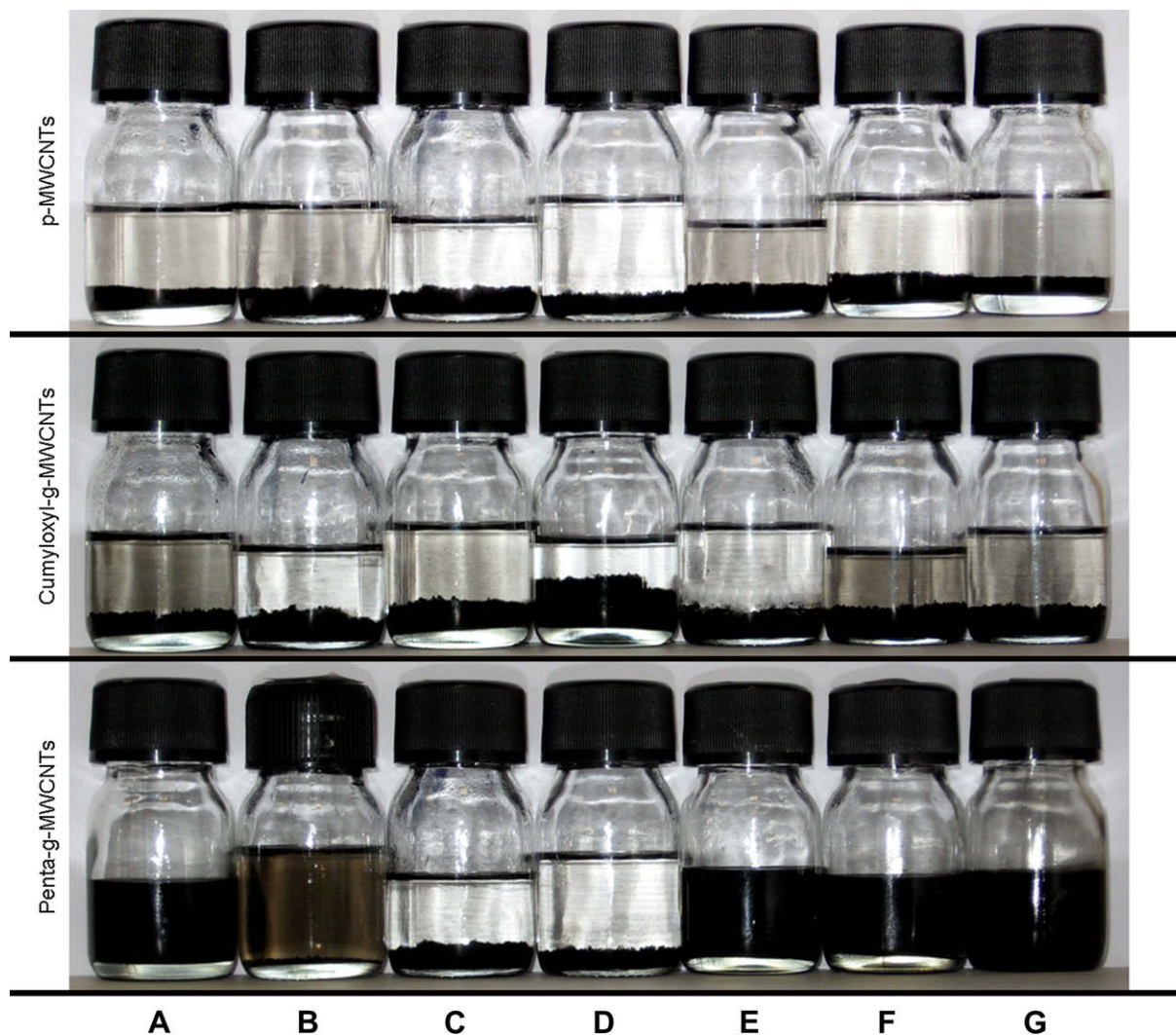
Fig. 6. Solubility behaviour of pristine carbon nanotubes (p-MWCNTs) after 5 min, cumyloxy grafted CNTs (cumyloxy-g-MWCNTs) after 30 min and pentadecane-grafted MWCNTs (penta-g-MWCNTs) after 2 months in DMF (A); acetone (B); chloroform (C); THF (D); toluene (E); DCB (F); xylene (G).
